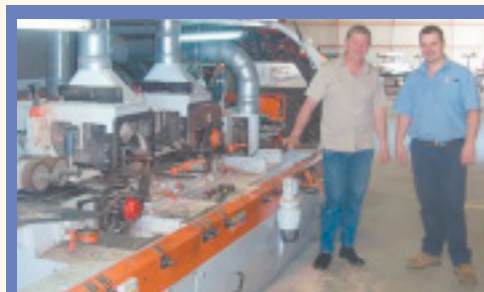
SCE's dedicated in-house Leadermac technician Daniel Coombes (right) stands beside Owen Jenkin, head machine operator at Whillands Sawmill in Victoria. Danny oversaw this installation featuring a 6-head plus universal Leadermac Hypermac moulder. Whillands produces a range of assorted hardwood products, including structural flooring.
