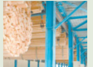
Each of these 40 sling sorter bays can hold an impressive 12,000kg.
