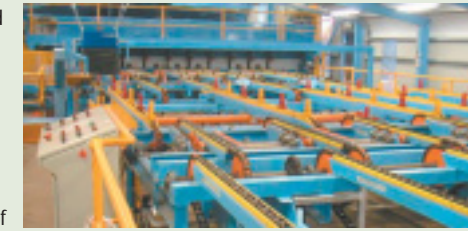
View of Sling Sorter from the infeed perspective.
