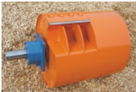
Chipper drum for large roundwood, with one half-length knife on each of the drum halves displaced 180 degrees against each other.
